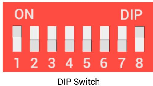
Generally, the ZCAN expansion module has an 8-code DIP switch to do communication configuration and resource mapping, dial ON to take effect, and the meaning of the DIP is as follows:
